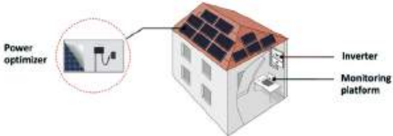
Figure 1: The SolarEdge power harvesting system components
