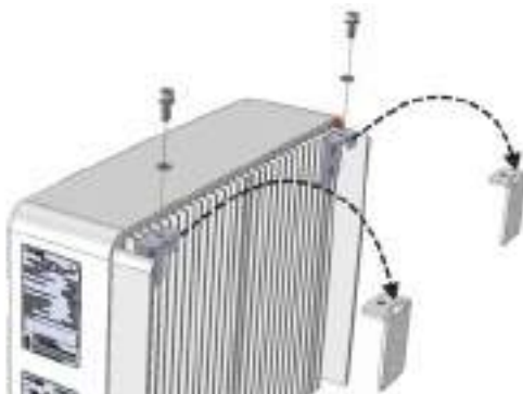
Figure 8: Hanging the inverter on the bracket
